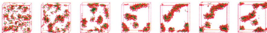
Plate 2 –DPD simulation of a system with less repulsive head group interactions. Predicted evolution of structure over 10,000 DPD time steps starting with a random distribution of surfactant molecules.
