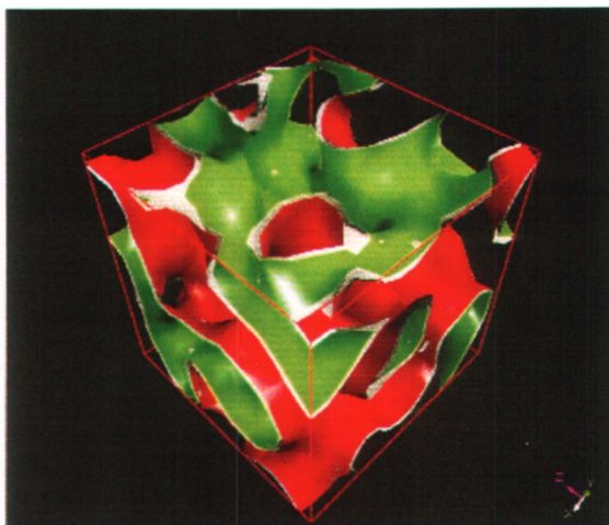
Plate 2a. Snapshot from MesoDyn simulation of polystyrene and polybutadiene equi-molar mixture. The surfaces indicate where each component falls to half its maximum density (unsurprisingly these surfaces coincide).
